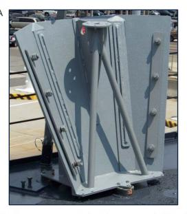
By utilizing a 20° deflection angle and "clean face" design, the BWS ensures maximum safety for security personnel by safely directing fragmentation down and away from the protected Sentry's position. This angle also reduces the Radar signature of the BWS when used aboard ship.
